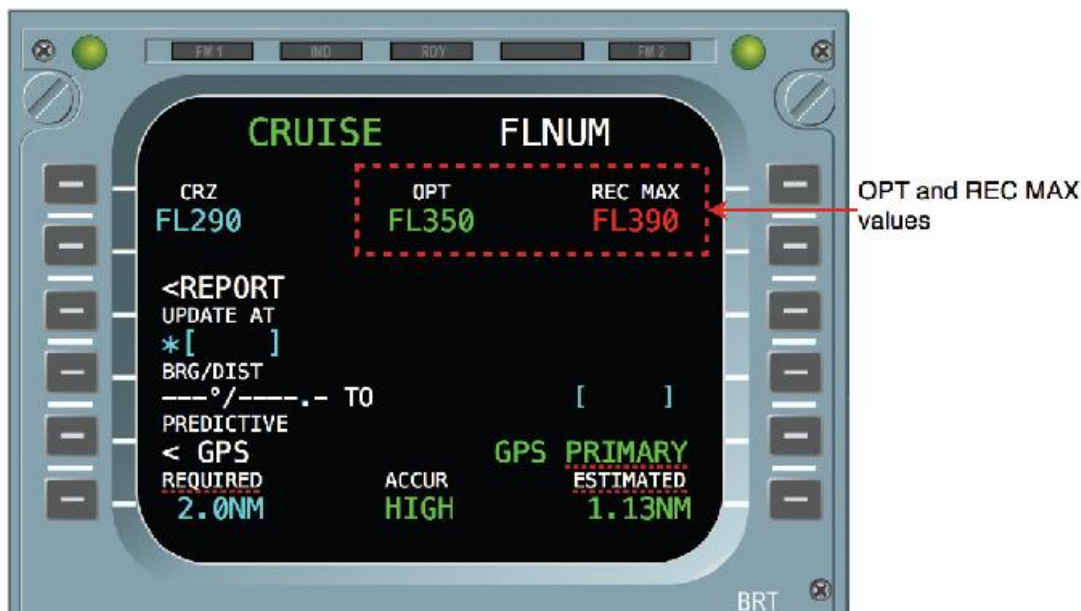
Figure 12: Example of a "PROG" page from FMS
