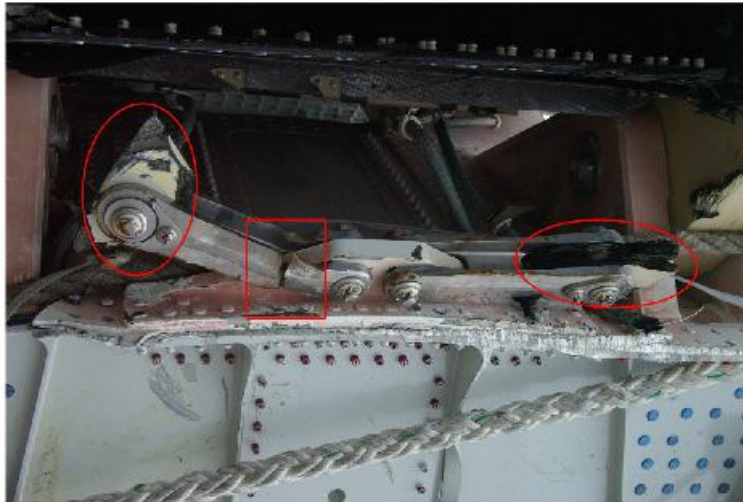
Figure 54: Compression failure of the aft spar at the level of the attachments of the lateral load pick-up rods and failure of the left-hand rod by buckling
