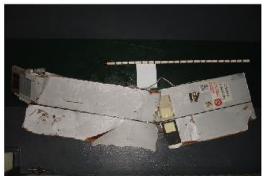
Figure 37: Metallic stiffeners deformed by buckling
