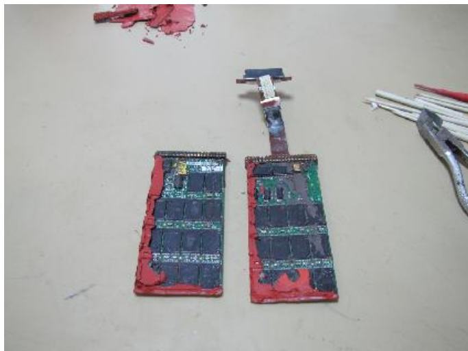
Figure 23: CVR memory boards before cleaning
