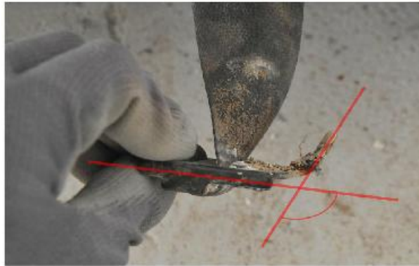
Figure 84: Malformation of the crotch belt fastening
