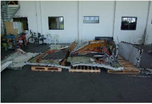
Figure 38: Floor of the LDMCR: with bottom-upwards deformation
