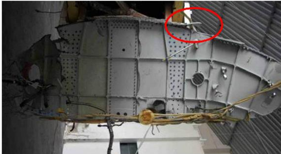
Figure 48: Frame 87: shearing of the frame and fuselage skin along the frame
