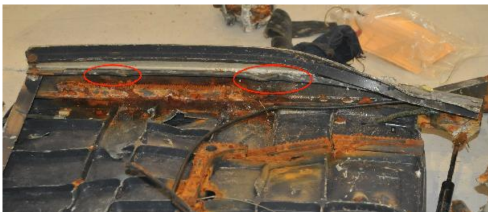
Figure 80: Roller marks on the guidance rail
