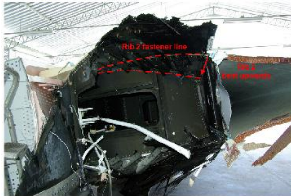
Figure 45: Rib 2 bent upwards as a result of bottom-upwards compression loads
