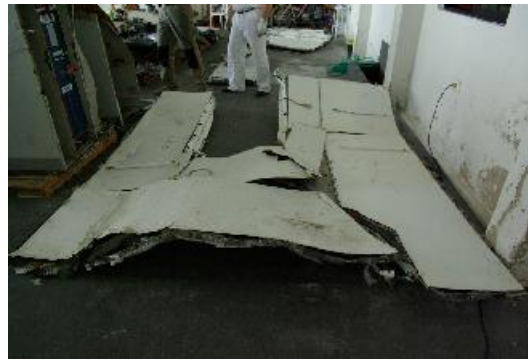
Figure 39: Ceiling of the LDMCR: with top-downwards deformation
